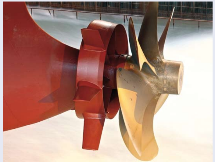
Becker Twisted Fin® installed on Santa Teresa in just three days
